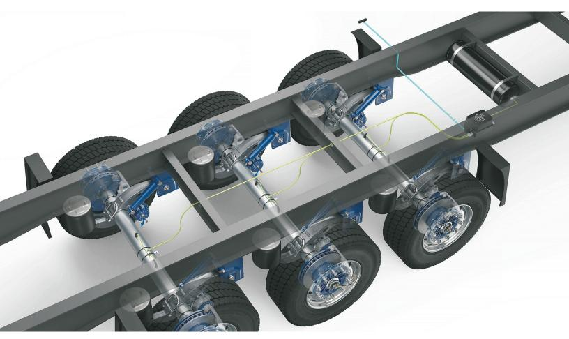
AirSave uses the existing trailer pneumatics and, with a fully automatic booster pump, ensures that the preset tyre pressure is maintained at all times.
