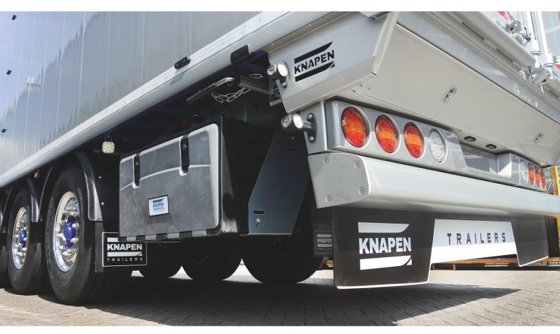
Knapen Trailers has adopted the new reinforced BPW air suspension ECO Air Compact HD for its moving floor trailers.
