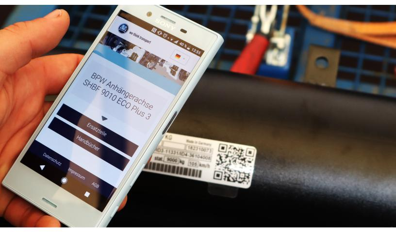
BPW now simplifies processes for workshops and vehicle operators with a new type plate, thereby making it easier to identify and order spare parts.
