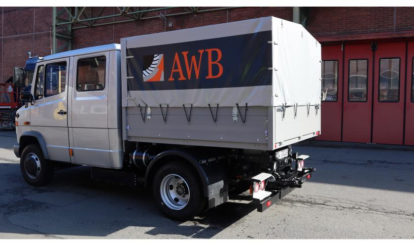
At bauma BPW will be presenting the options available for conversion with the eTransport electric drive axle on the AWB Köln company's Mercedes-Benz Vario with special bodywork.
