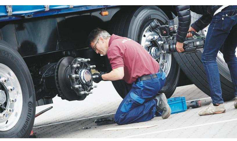
The ECO Disc brake produced by BPW allows brake service in record time. (Source: BPW Bergische Achsen KG)
