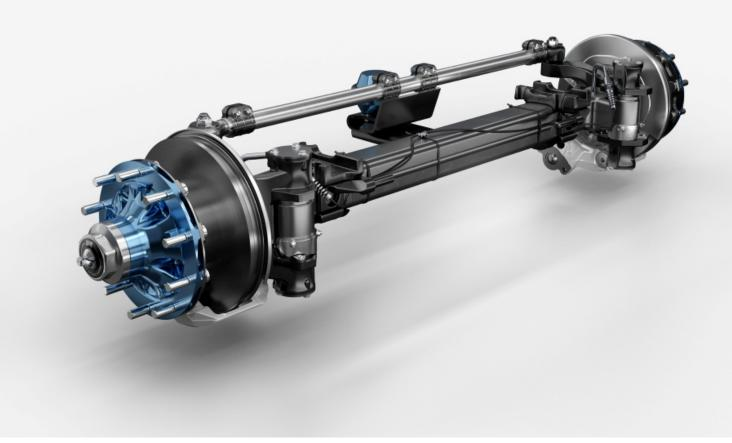
AirSave mounted on a BPW steering axle.
