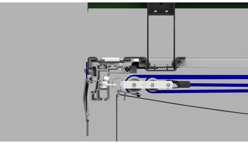
The MultiMaster is a multifunctional roof rail for the HESTAL sliding roof, which supports the roof and serves as an attachment for side tarpaulins, wall and support elements.
