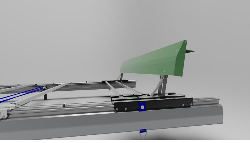
The aerodynamically optimised end beam promises to significantly increase efficiency in commercial vehicle traffic.
