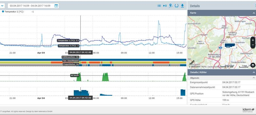
cargofleet 3 gives a quick overview of the fleet and individual functions – the screenshot shows the temperature profile of a refrigerated semitrailer.
