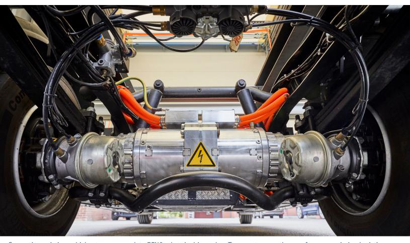
Converting existing vehicles to accommodate BPW's electric drive axle, eTransport, paves the way for zero-emission logistics.
