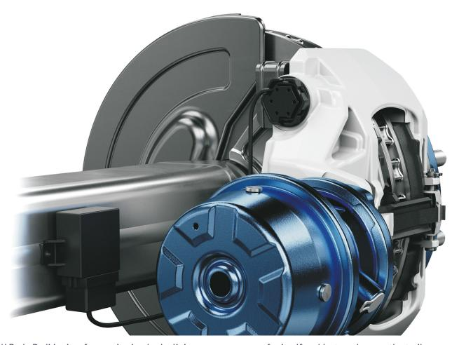
The BPW BrakePadMonitor for monitoring brake lining wear soon pays for itself and lasts as long as the trailer.
