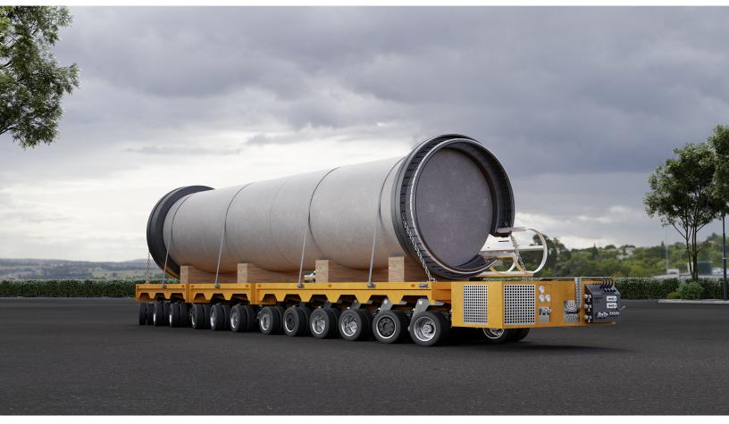
Modular vehicles move extreme loads under challenging conditions. One transport module is equipped with two to eight axle lines or with four to 16 pendulum axles.
